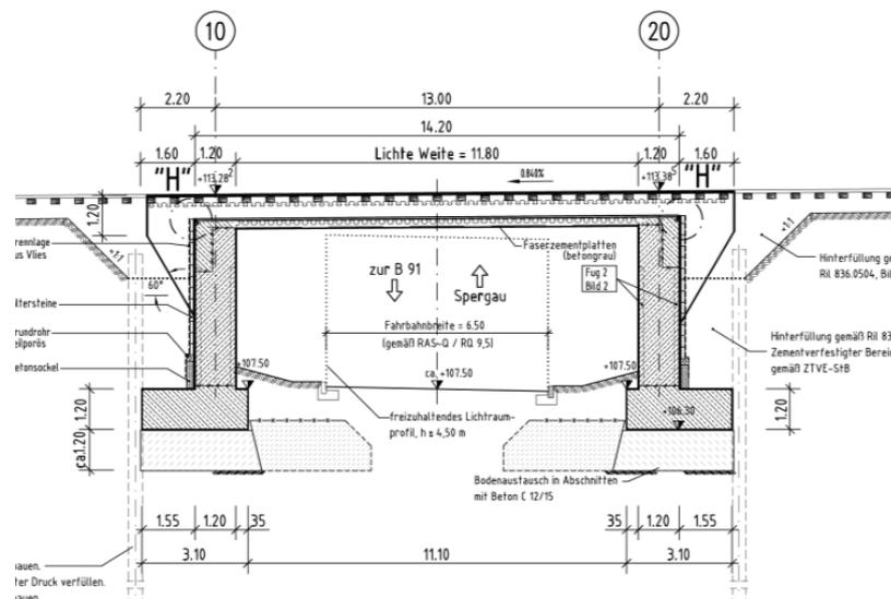
Figure 127 - Longitudinal section railway crossing over K2174 (Maienweg) in Leuna
