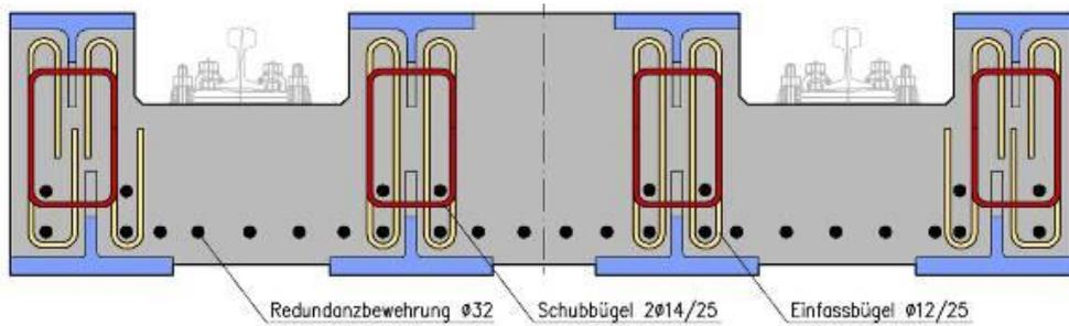
Figure 6 - Schematic reinforcement for the cross-section
