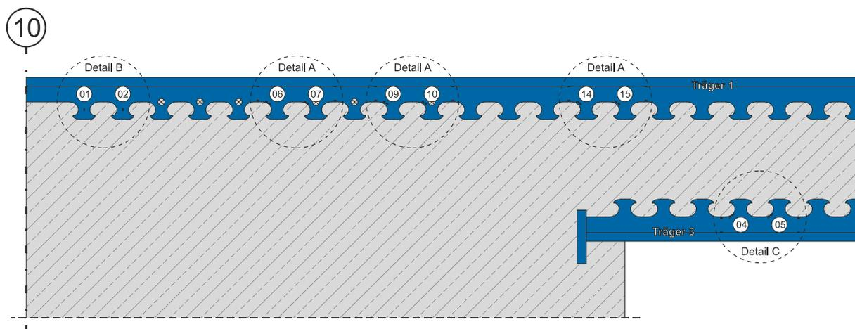
Figure 86 - Measurement sections at superstructure (axis 10)
