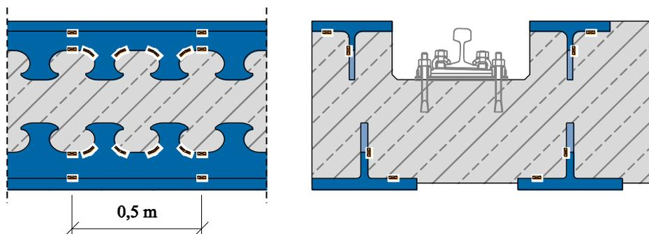
Figure 76 - Position of strain gauges
