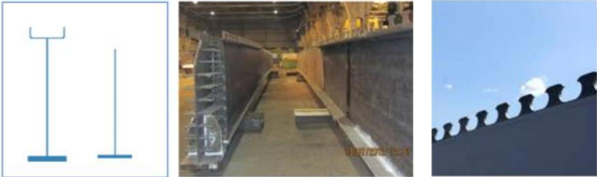
Figure 94 - The steel girder type sections; Steel girders in the workshop; the cutting line geometry of the composite dowels.
