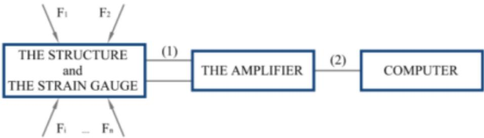
Figure 102 - The principle of the strain gauge chain used for the probes.
