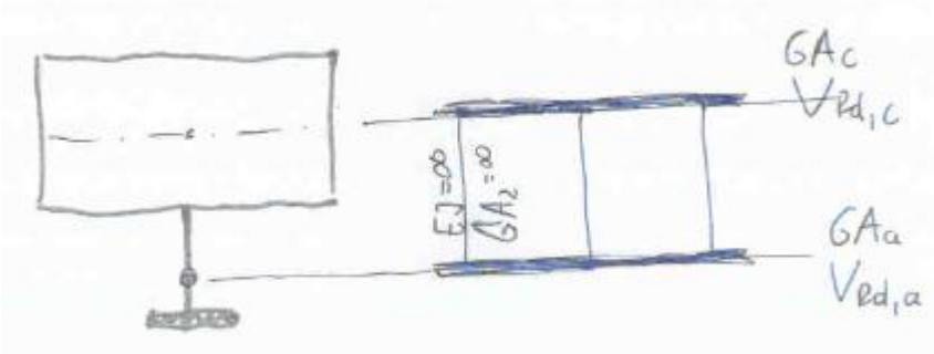
The point is how to dimension such sections for vertical shear, especially how to design stirrups in thick concrete plate. Reinforcing system is very safe in PE4 because aware of this idea we had to over dimension it – in future (if problem solved and design formulas established) a big reduction of stirrups can be expected for such structures. Important aspect of thick plate is big torsional stiffness what improves cooperation between girders.
