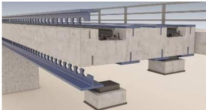
Figure 4 - Application of VFT-Rail Cross-Sections using PreCoBeam technology
