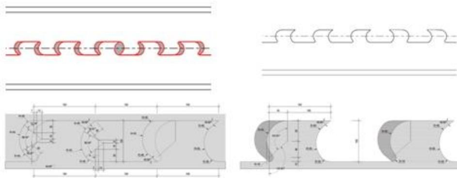
Figure 47 - Execution details of the steel girders, geometry of the steel dowel
