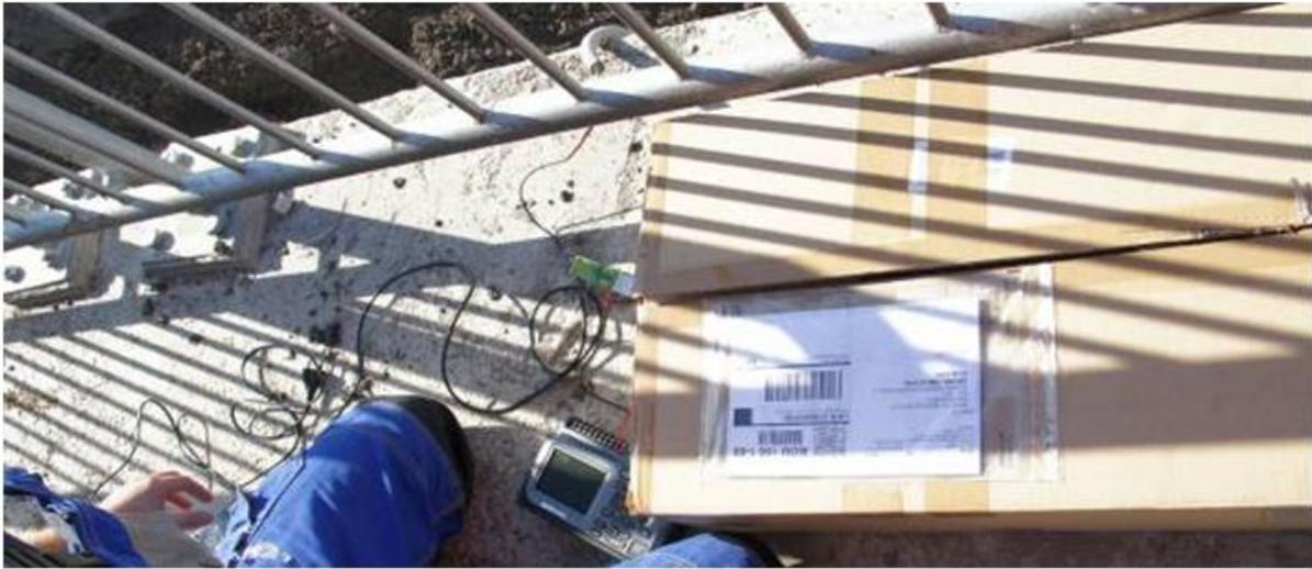
Figure 103 - Displacement transducer device
