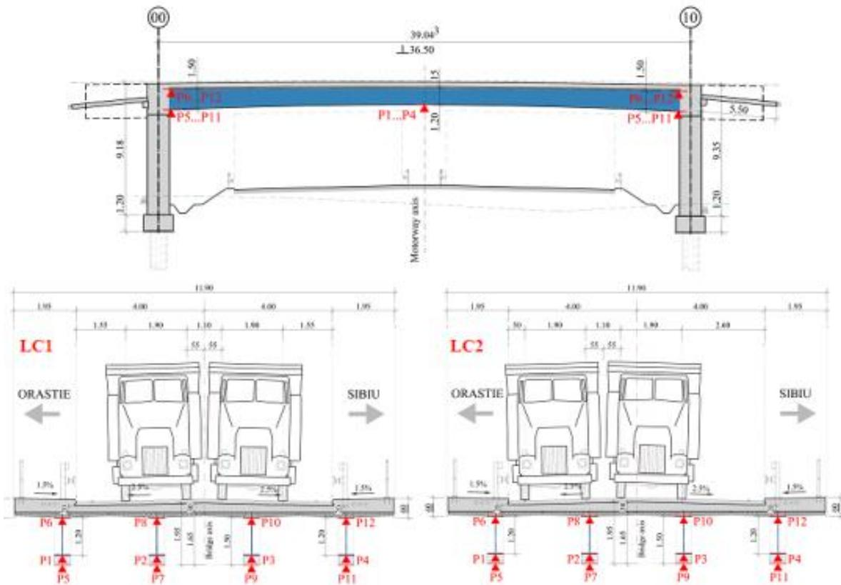
Figure 108 - The read points for the static / dynamic test schema, load schema 1 – LC1 and load schema 2 – LC2.
