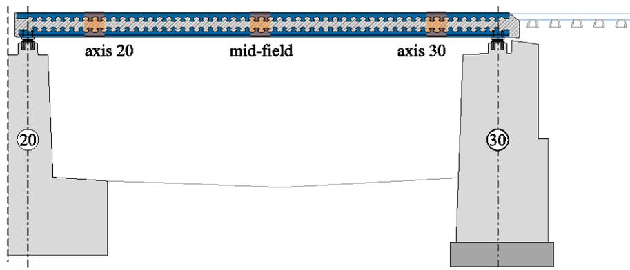
Figure 75 - Measurement sections at superstructure between axis 20 and axis 30
