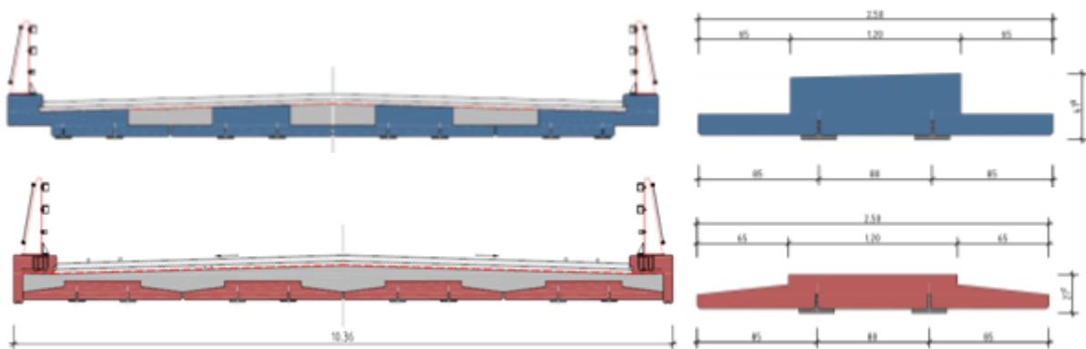
Figure 41 - General new cross sections and details with the precast elements
