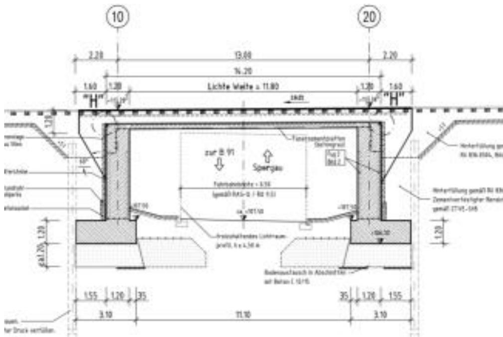
Figure 83 - Longitudinal section railway crossing over K2174 (Maienweg) in Leuna
