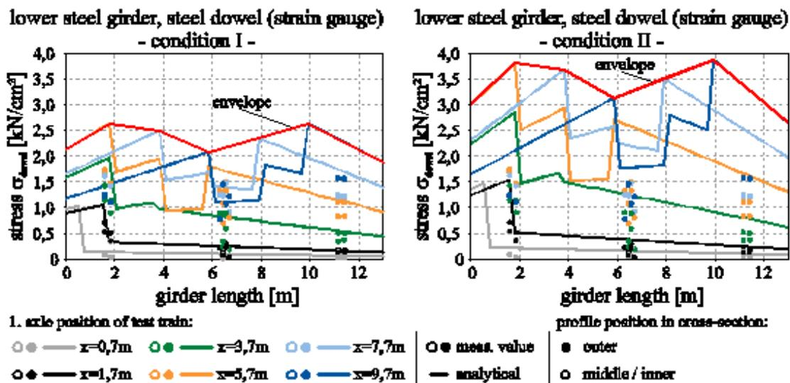
Figure 81 - Measured strains / stresses within the region of the hot-spot, lower external reinforcement, compared to calculated values for condition I (left) and condition II (right)
