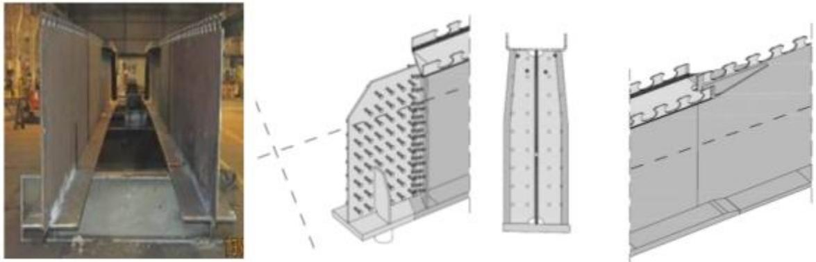
Figure 95 - The steel girder type sections; the end steel girders detail and the transition detail between the two types of section.
