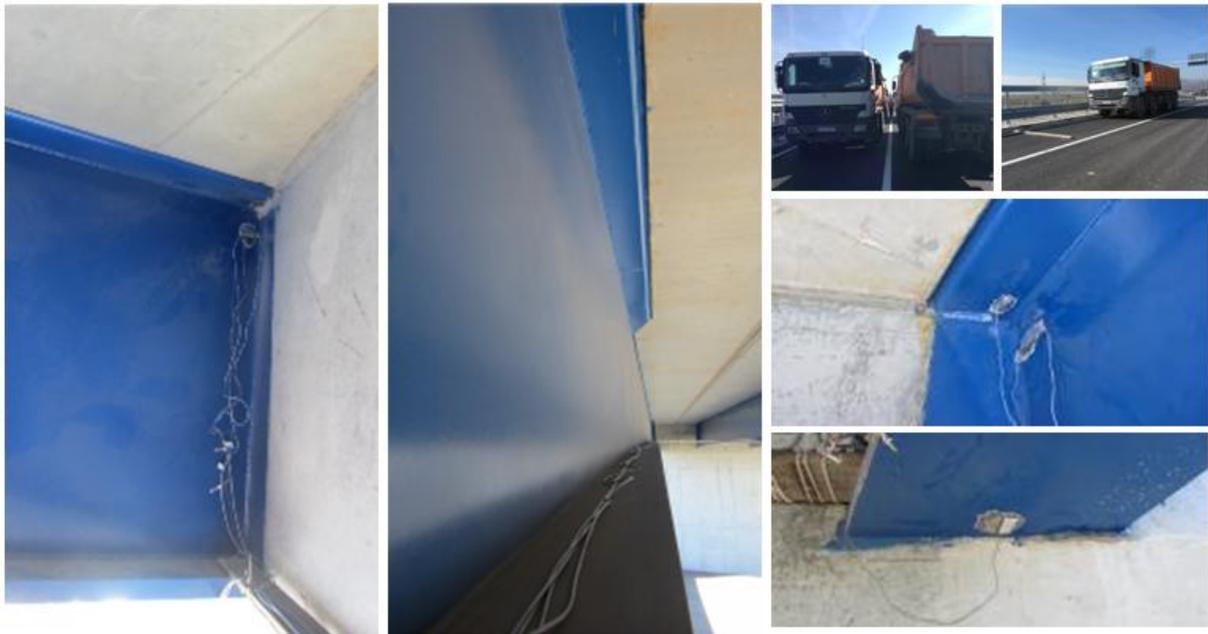
Figure 99 - Installed strain gauges on the section of the bridge in the in-situ test day
