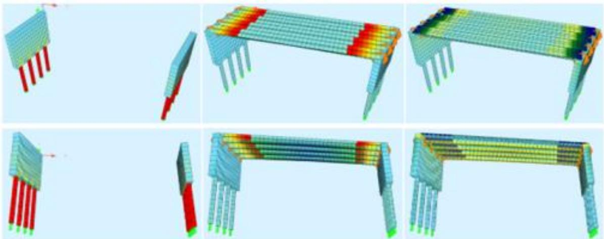
Figure 104 - Construction stage manager steps
