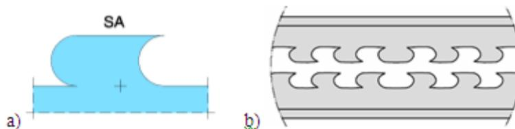
Figure 45 - SA or fin shaped steel dowels: The SA shape (a), Direction change of the composite dowels in the middle of the girder (b)
