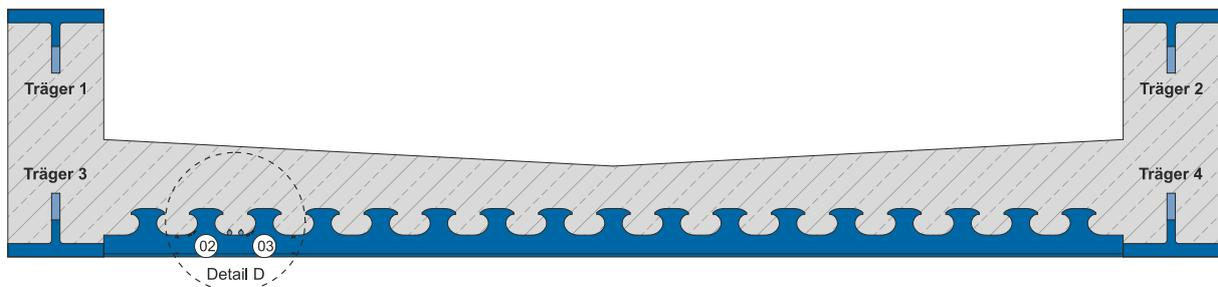
Figure 84 - Cross section VFT-Rail with composite dowels and composite slab
