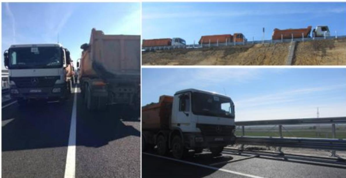
Figure 98 - MAN TGA convoy – front view, lateral view; dynamic load test MAN TGA vehicle.
