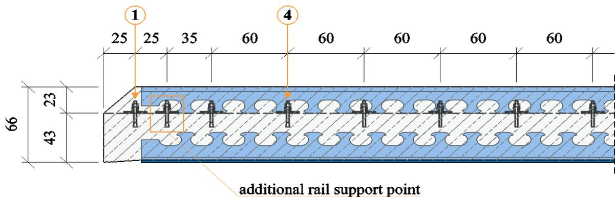
Figure 63 - Pattern of rail fasteners at the end of superstructure
