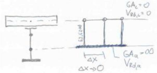
This is classic concrete section expressed by Vierendeel beam (concrete part alone takes vertical shear force):
