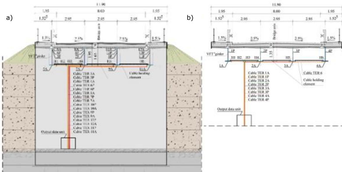
Figure 101 - Installed strains on the section of the bridge; a) Cross section on the supports area; b) Cross section on the field.
