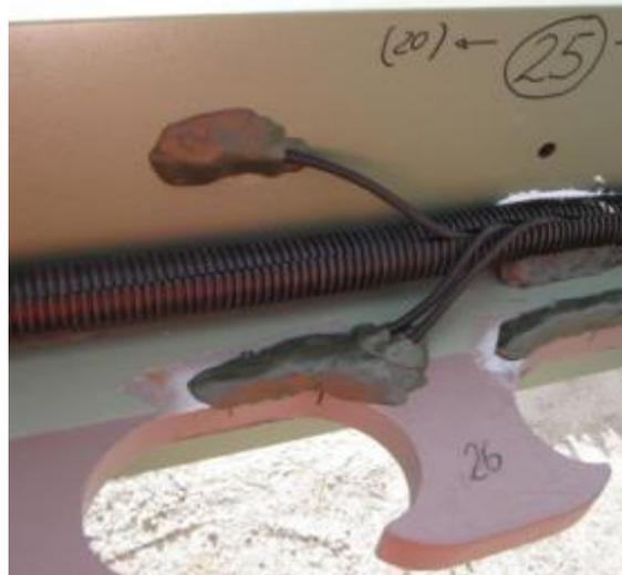
Figure 77 - Protected strain gauges, covered with 2-component adhesive (PS-adhesive) and permanent elastic cement (AK22)
