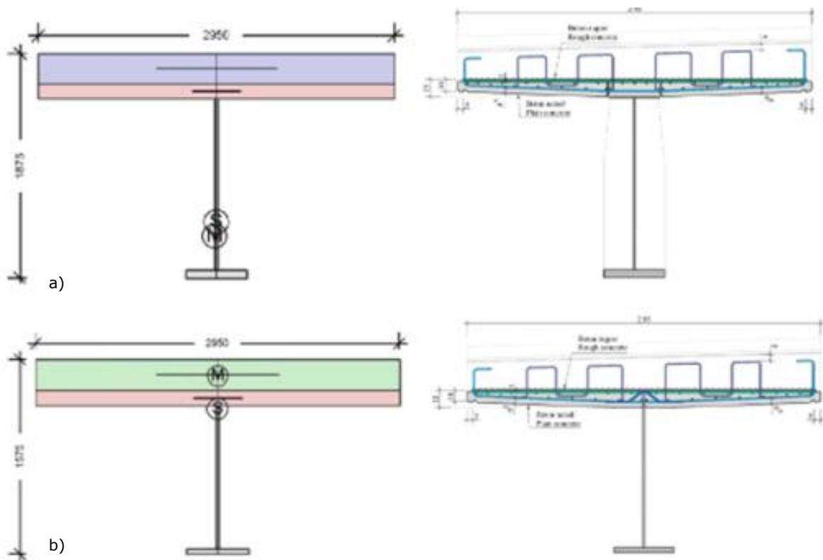
Figure 105 - a) Cross section of the supports area; b) Cross section of the field.
