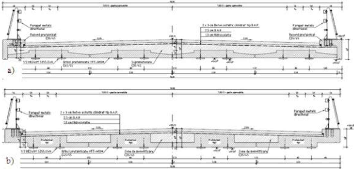
Figure 39 - General cross section: Solution 1 (a), Solution 2 (b)
