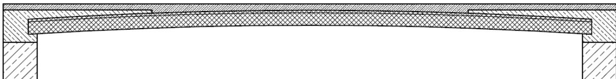
It enables optimisation of composite girder by modification of reinforced concrete body and with constant steel profile. With increasing thickness of concrete plate it leads to quite new problem of "steel beam with thick concrete plate" what is presented in separate point.
