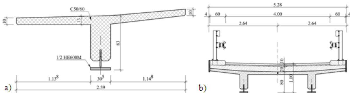
Figure 46 - VFT-WIB – mono-WIB cross section (a), Superstructure cross section (b)
