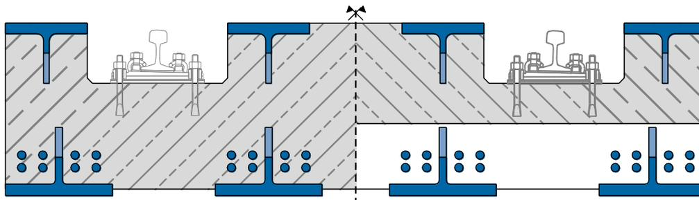
Figure 74 - Cross section for condition I (left) and condition II (right), rail support point drawn in for illustration purposes only
