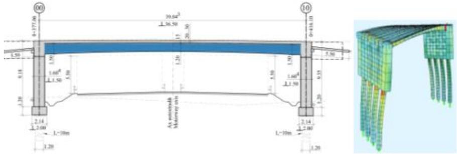
Figure 89 - Left: longitudinal section, Right: design model
