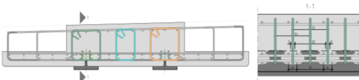
Figure 42 - Reinforcement detail of the precast composite girder
