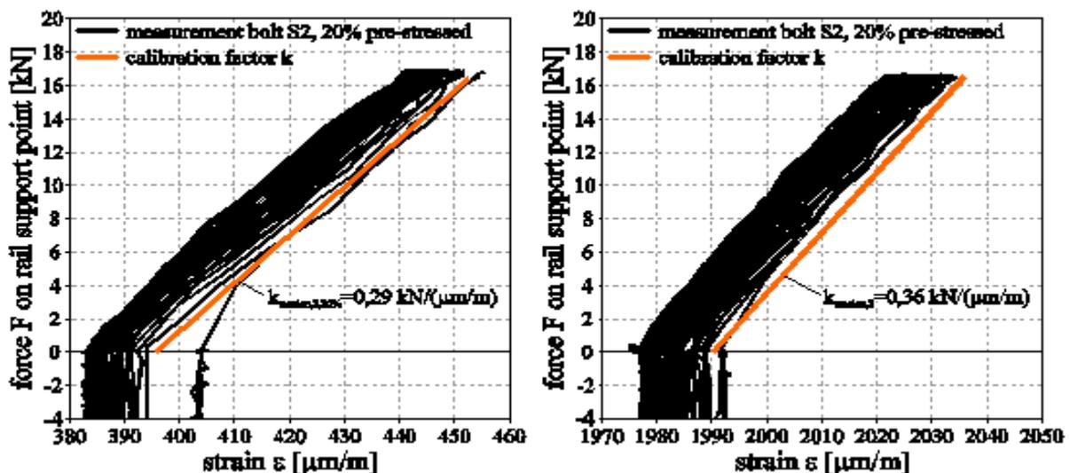
Figure 71 - Strain change in measurement bolt S2 depending on applied force (20% pre-stressed, 100% pre-stressed)
