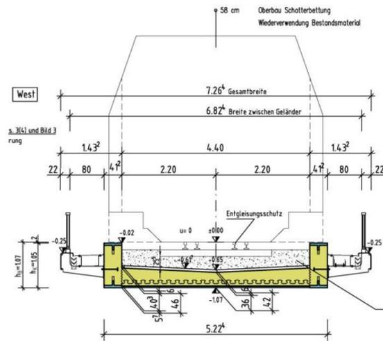
Figure 131 - Leuna Bridge: Cross section
