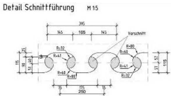
Figure 7 - Detailed cutting-geometry
