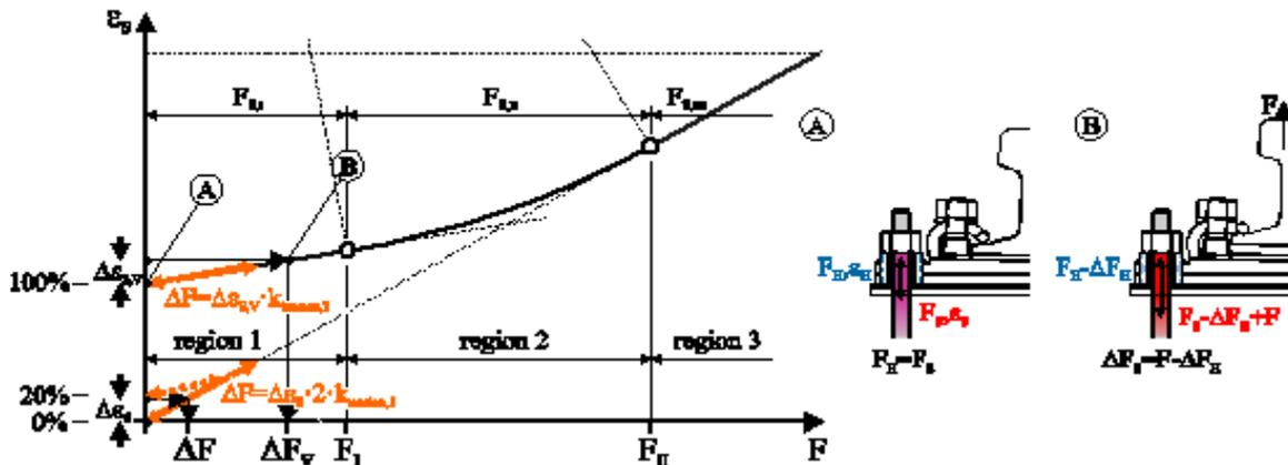
Figure 72 - Bolt force function: measured strain  $\Delta\epsilon_s$  over jack force  $\Delta F$  at rail support point
