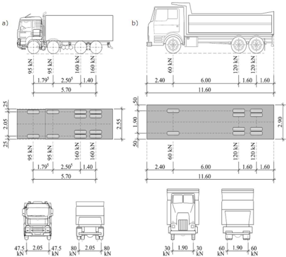
Figure 97 - a) A30 convoy – lateral view, plan view, front / back view;
