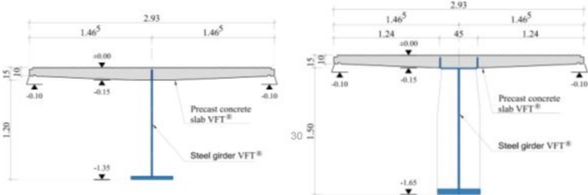
Figure 91 - The formwork cross section of the Prefabricated Composite Girder VFT®
