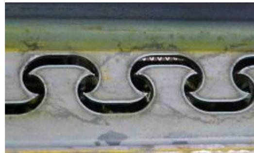
Figure 8 - Dowels after cutting-process
