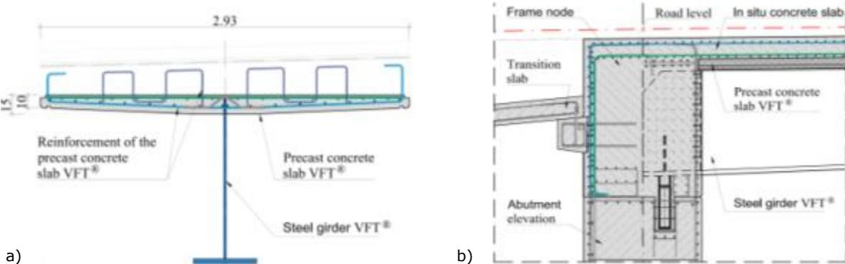
Figure 92- a) Reinforced cross section of the Prefabricated Composite Girder VFT®, b) Frame node reinforcement detail
