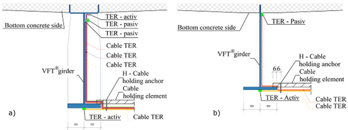
Figure 100 - Installed strains on the section of the bridge; a) Cross section of the supports area; b) Cross section of the field.
