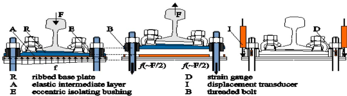
Figure 66 - Load bearing mechanism of rail support point ECF (principle, superelevated illustration), measurement equipment at rail support point ECF (principle)
