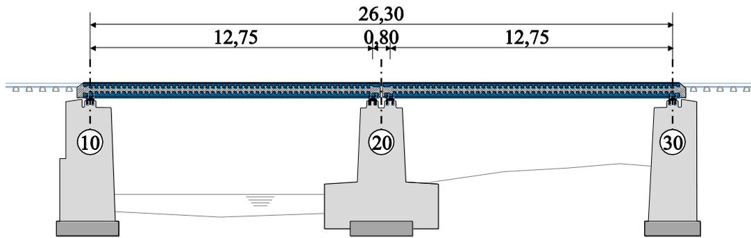
Figure 61 - Longitudinal section railway crossing over the river "Simmerbach" with two VFT-Rail® girders, placed on toughened sub-structure
