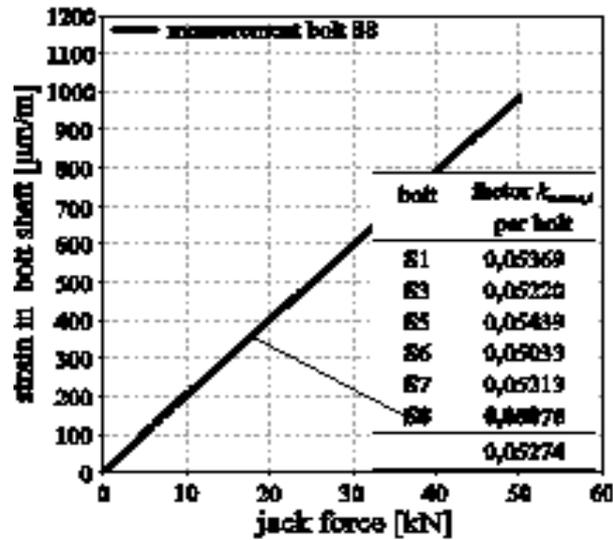
Figure 68 - Calibration of measurement bolts (here: measurement bolt S8), conversion of strain in measurement bolts into pre-tension force
