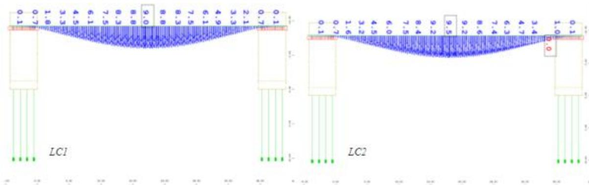
Figure 110 - Vertical displacement diagrams – test load schema 1 – LC1 and load schema 2 – LC2
