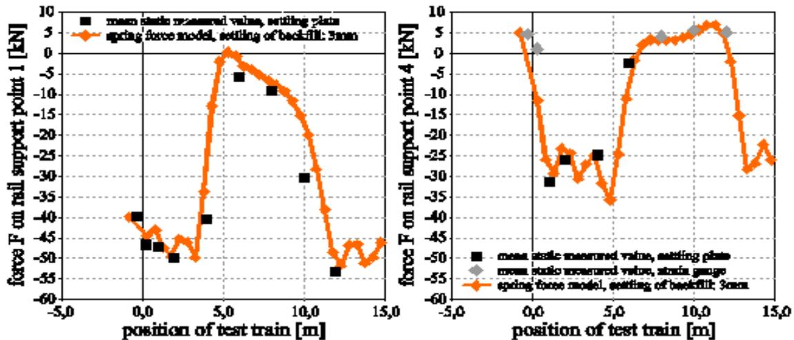
Figure 73 - Compression force / tension force acting on controlling rail support points 1 (left) and 4 (right), caused by static loading (test train)
