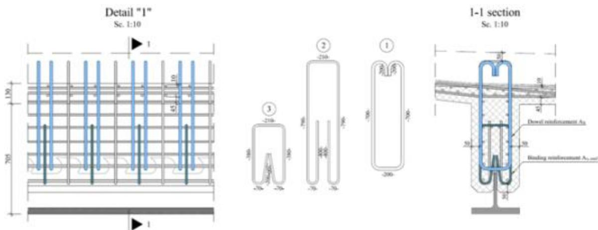
Figure 48 - Composite dowels – reinforcement details
