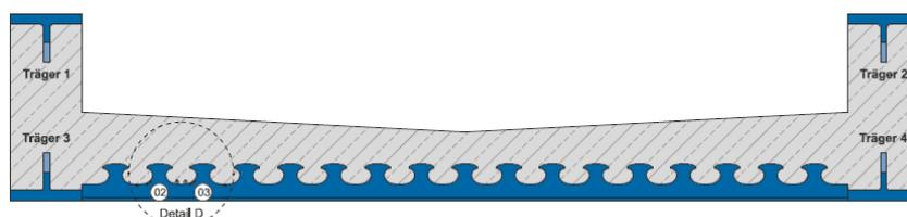
Figure 128 - Cross section VFT-Rail with composite dowels and composite slab
