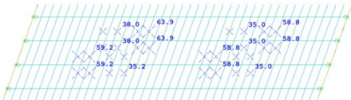
Figure 107 - The load test vehicles designed in the FEM model
