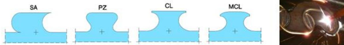
Figure 44 - Cutting line types: fin (SA), puzzle (PZ), clothoidal (CL), modified clothoidal (MCL)
