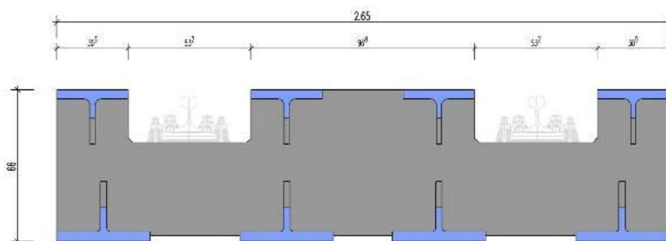
Figure 5 - VFT-Rail cross-section with 66cm construction height and external reinforcement
