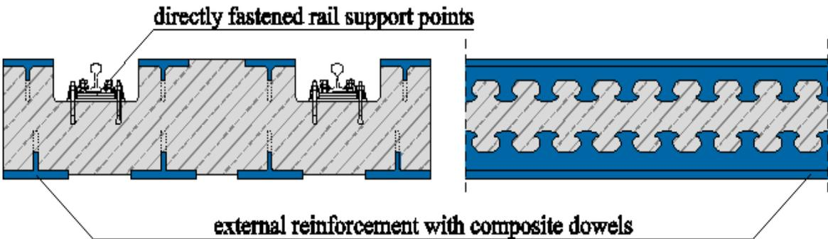
Figure 60 - Transverse cross section (left) VFT-Rail® with rail support points directly fastened to the superstructure and composite dowel and longitudinal cross section (right, depicting the clothoidal shape of the dowels)
