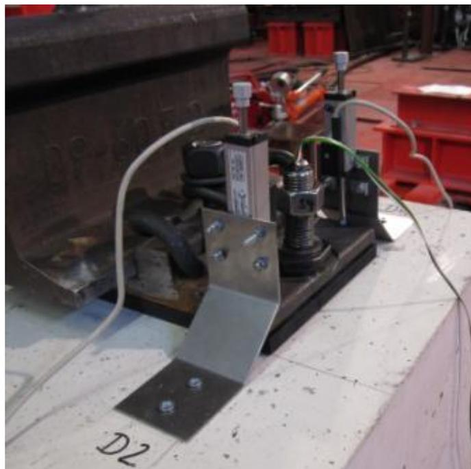
Figure 69 - Test set-up with measurement devices (unstressed measurement bolt S4 and displacement transducers W2, W4)
