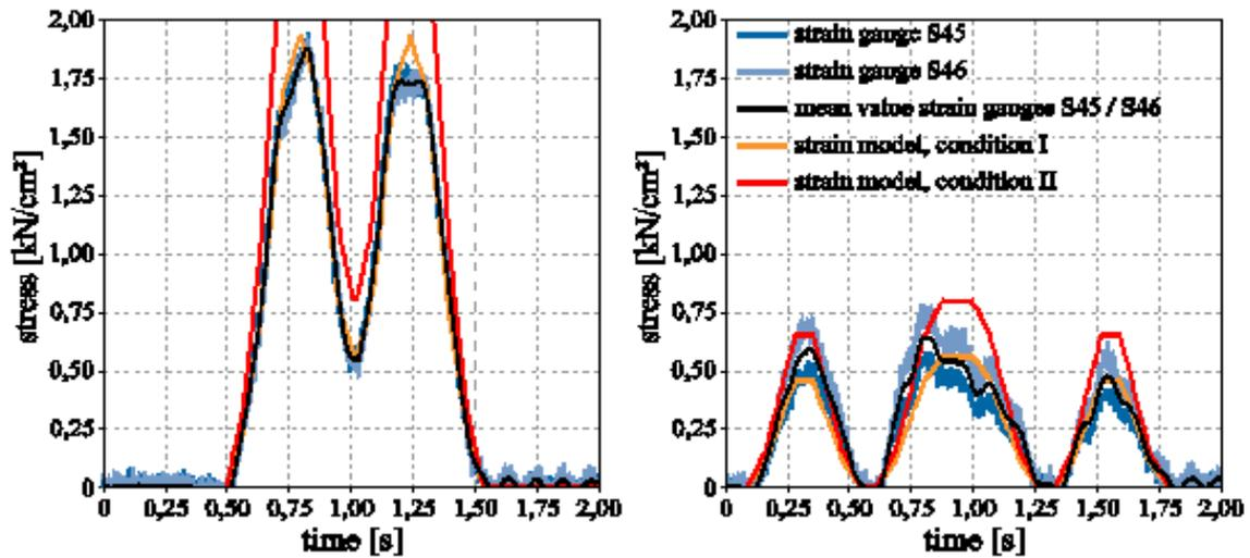
Figure 82 - Stresses in lower flange caused by crossing of test train (100 km/h, left) and regional train (120 km/h, right)
