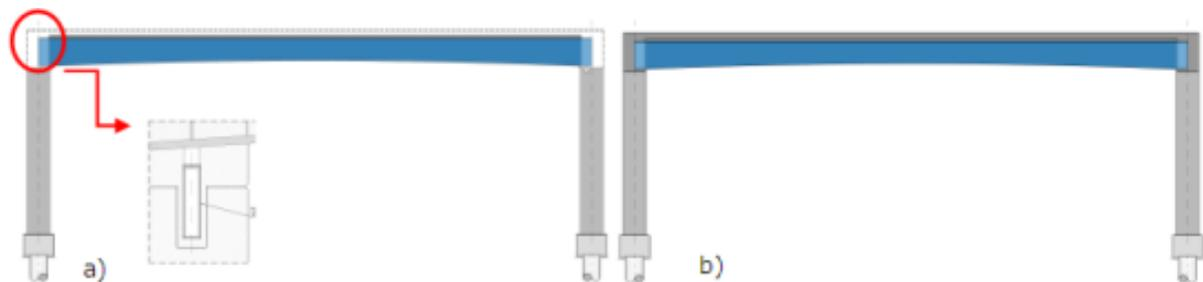
Figure 106 - Construction stages: a) Simple supported girder; b) Frame effect
