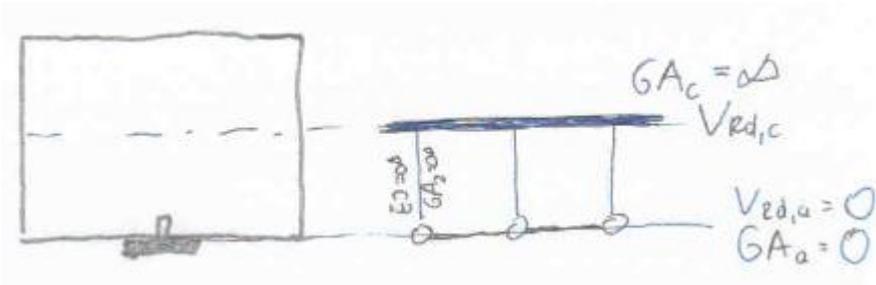
This is "general" composite section expressed by Vierendeel beam (vertical shear force is handled by steel and concrete parts acting together depending on their geometries and internal lever arm – see annex):
