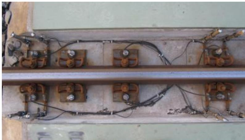
Figure 67 - Measurement devices for monitoring of forces acting on rail support points (1<sup>st</sup>, 2<sup>nd</sup> and 4<sup>th</sup> rail support point equipped)
