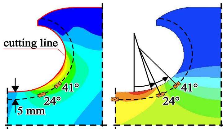
Figure 78 - Calculated stress distribution (schematic, left: local loading due to shear force acting at steel dowel, right: global loading due to axial deformation of the external reinforcement due to bending of the composite section) [P804]
