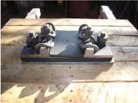
Figure 12 - Rail support before mounting
