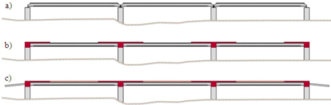
Figure 49 - Superstructure construction phases: laying of the VFT-WIB composite girders in their final position (a), frame node and end sections of the deck concreting (b), deck concreting (c)
