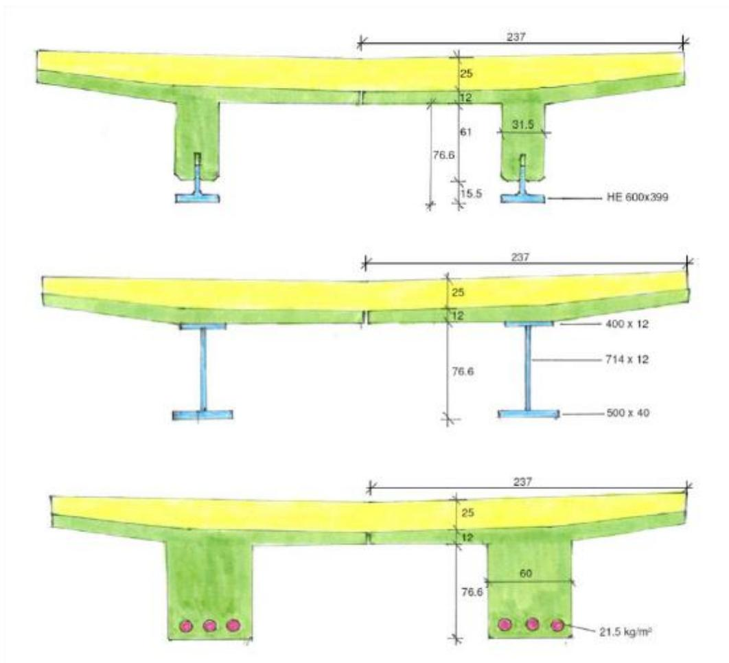
Figure 120 - Dimensions of Preco-Beam girders for Vigaun-Bridge and of preliminary design for VFT and pre-stressed girders
