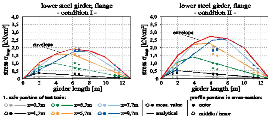
Figure 79 - Measured strains / stresses on the inner side of the flange (lower external steel girder, points) compared to calculated stresses for condition I (left) and condition II (right)
