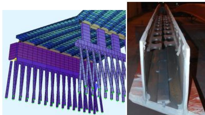
It was a lot of effort at design stage. And due to tolerances we decided to use welding on site and to use additional plates between steel girders to connect them together. This was better solution than screws usually used if straight girders but it was a problem at construction site to weld because of lack of space (dense reinforcement of crossbeams).
