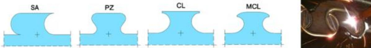
Figure 126 - Cutting line types: fin (SA), puzzle (PZ), clothoidal (CL), modified clothoidal (MCL) [8].
