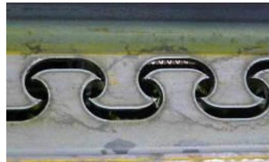
Figure 8 - Dowels after cutting-process
