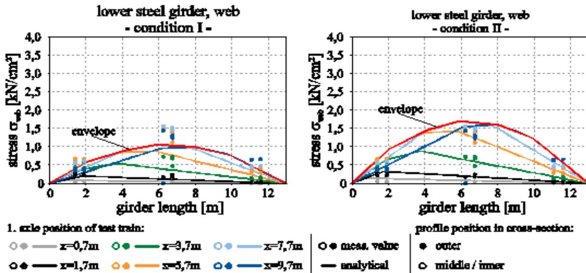
Figure 80 - Measured strains / stresses at web of lower external reinforcement, compared to calculated values for condition I (left) and condition II (right)
